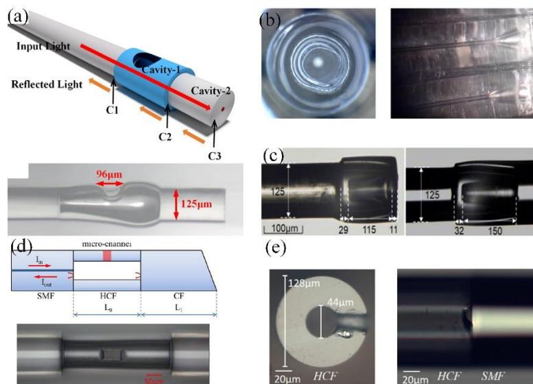
**Fig. 3** (a)–(e) Optic-fiber FP pressure sensor made by laser processing technology.
