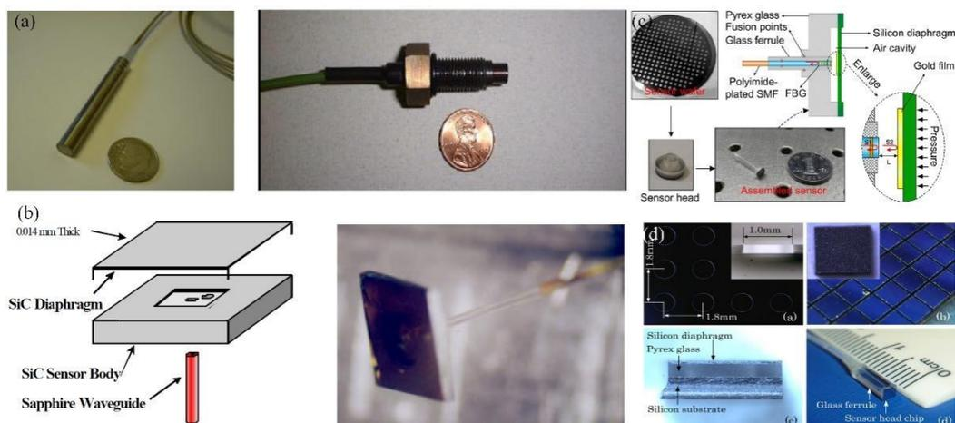
**Fig. 6** (a)-(b) Optic-fiber FP pressure sensor based on Si and SiC developed by Luna Company
