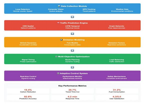
The Emission Modeling Component implements physics-based vehicle dynamics models enhanced with machine learning techniques to accurately estimate carbon emissions based on microscopic traffic characteristics including acceleration profiles, fuel consumption rates, and
