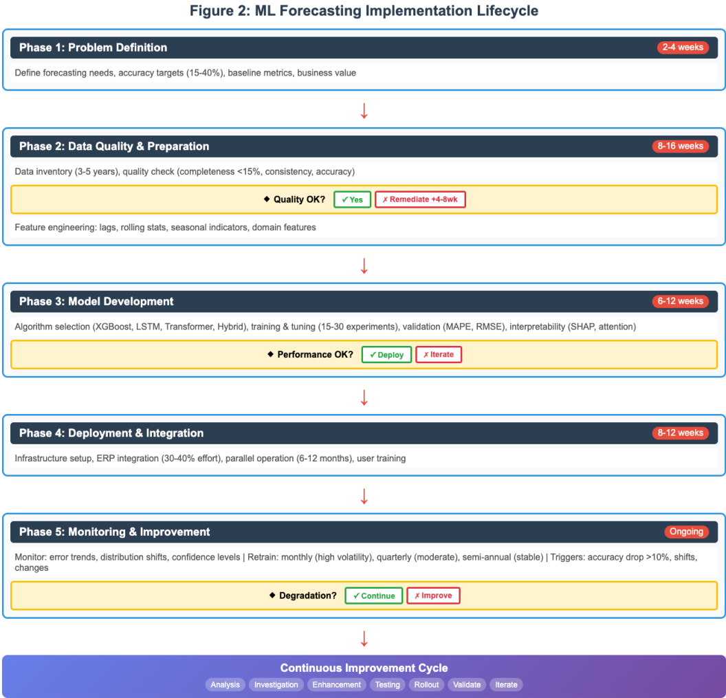
Figure 2 : ML forecasting implementation lifecycle workflow showing progression from problem definition through data quality assessment, model development, deployment, and continuous improvement with drift detection and retraining triggers.
